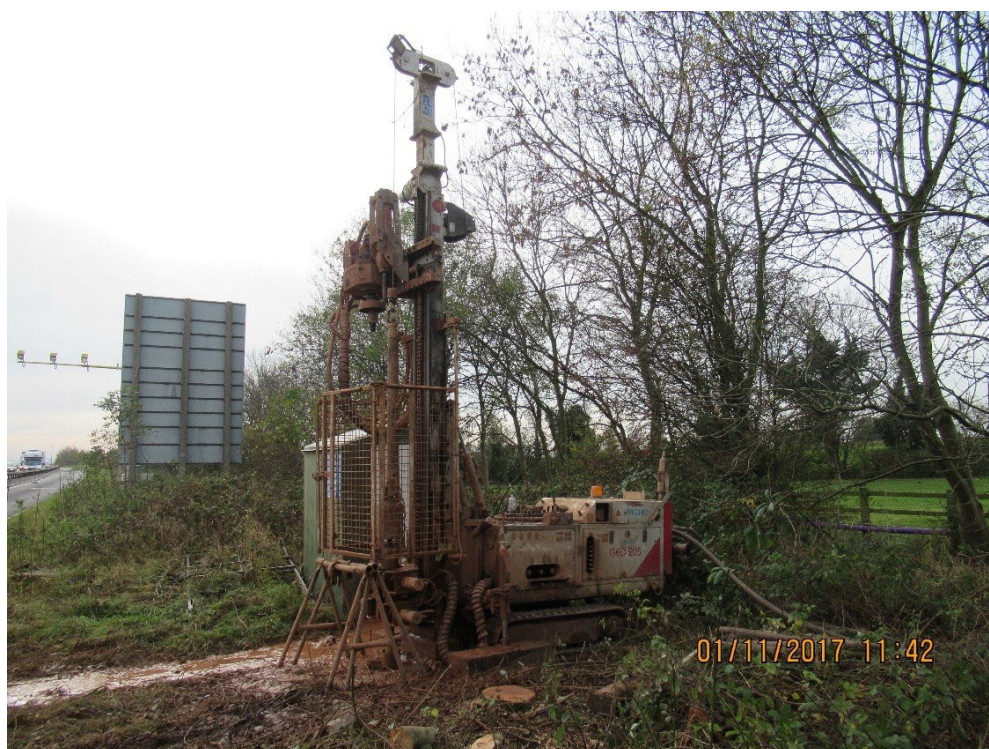
Figure 10-1 Dynamic sampling rig Link 4b NB ch 192900 (pulled onto verge during day shift)
