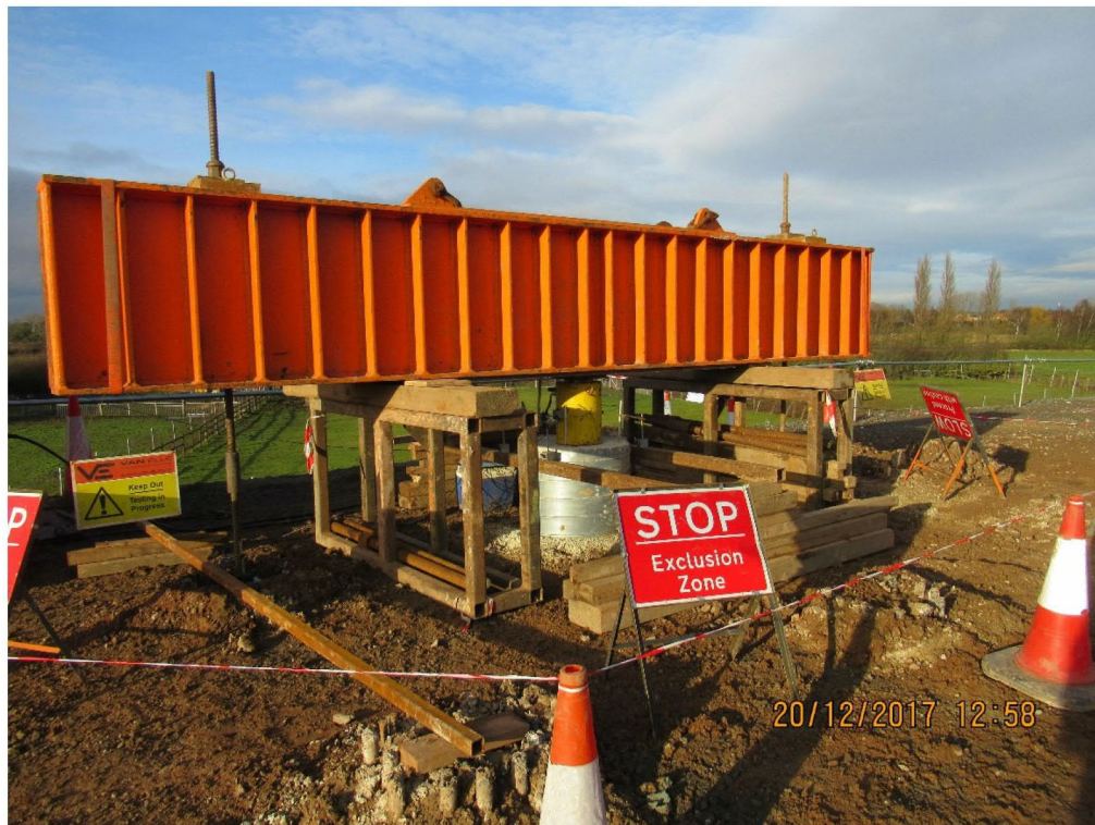
Figure 12-1 Static load test on 0.75m diameter pile: Gantry 313 (Link 4b NB)
