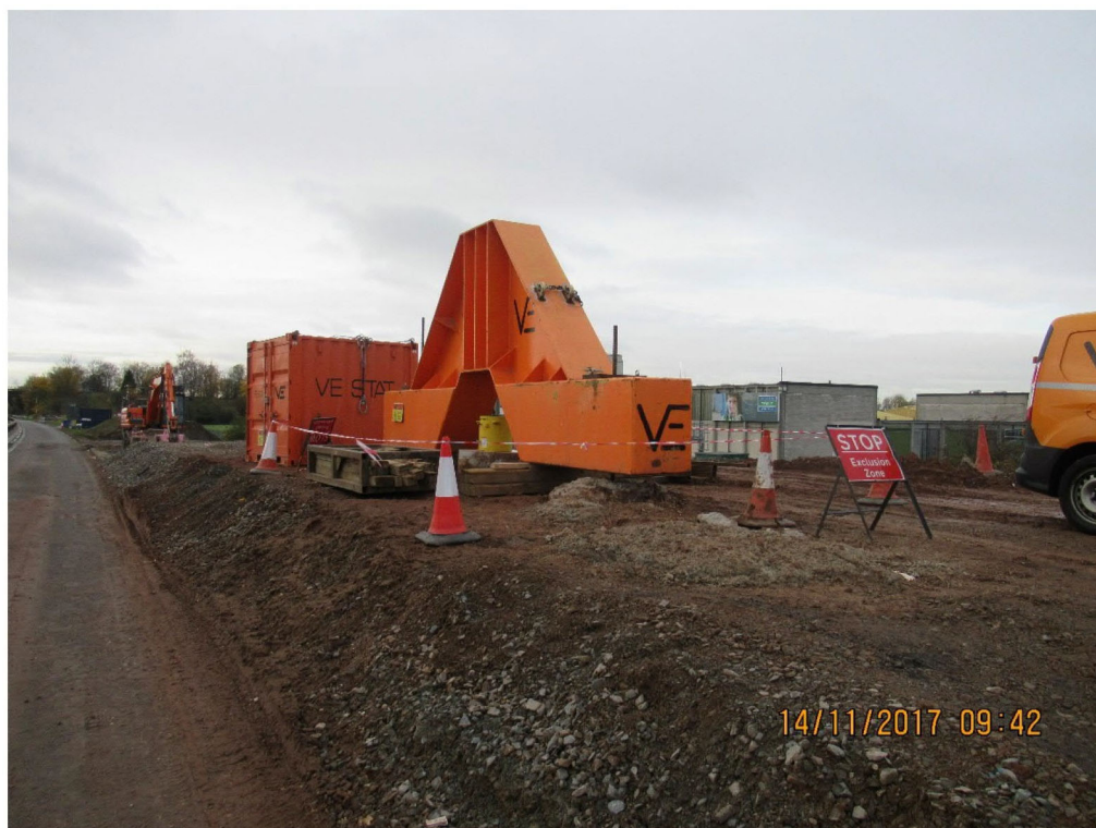
Figure 12-2 Static load test on 0.9m diameter pile: Gantry G311 Link 4b NB
